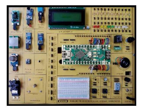
This trainer has been designed with a view to provide practical and experimental knowledge of Internet of Things (IOT) with Sensors programing with Arduino Nano IOT Board.
