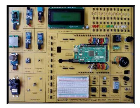
This trainer has been designed with a view to provide practical and experimental knowledge of Internet of Things (IOT) with Sensors programing with Arduino Due IOT Board.
