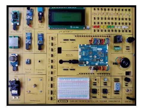
This trainer has been designed with a view to provide practical and experimental knowledge of Internet of Things (IOT) with Sensors programing with Arduino Zero IOT Board.
