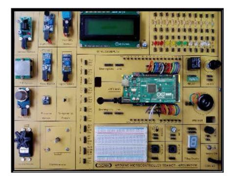
This trainer has been designed with a view to provide practical and experimental knowledge of Internet of Things (IOT) with Sensors programing with Arduino GIGA IOT Board.
