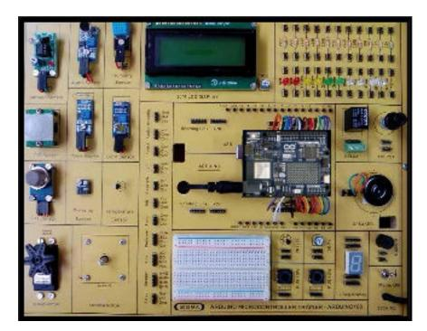
This trainer has been designed with a view to provide practical and experimental knowledge of Internet of Things (IOT) with Sensors programing with Arduino Wifi IOT Board.
