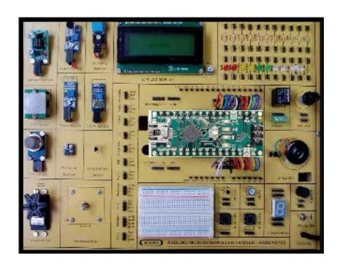
This trainer has been designed with a view to provide practical and experimental knowledge of Internet of Things (IOT) with Sensors programing with Arduino Nano ESP32 IOT Board.
