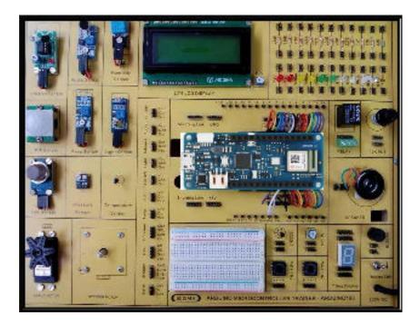
This trainer has been designed with a view to provide practical and experimental knowledge of Internet of Things (IOT) with Sensors programing with Arduino MKR1010 Wifi IOT Board.
