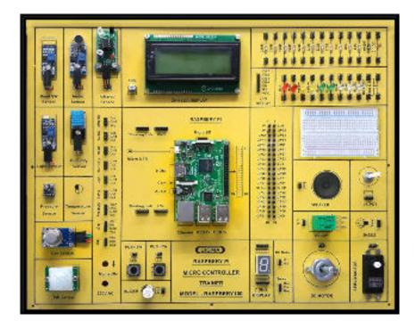
This trainer has been designed with a view to provide practical and experimental knowledge of Internet of Things (IOT) with Sensors programing with Raspberry IOT Board.
