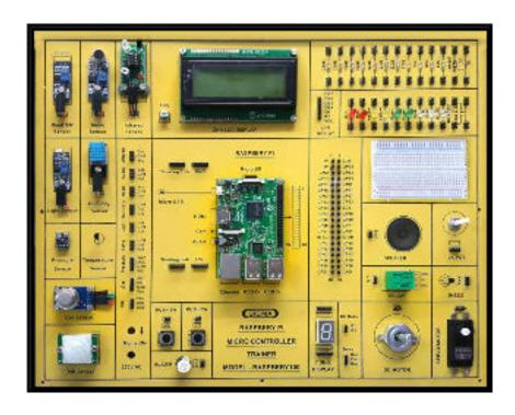
This trainer has been designed with a view to provide practical and experimental knowledge of Internet of Things (IOT) with Sensors programing with Raspberry Pi 5 IOT Board.
