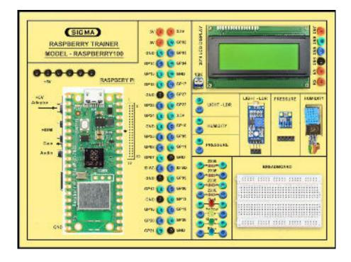
This trainer has been designed with a view to provide practical and experimental knowledge of Internet of Things (IOT) with Sensors programing with Raspberry PICO W Microcontroller Board.
