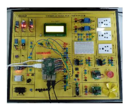
This trainer has been designed with a view to provide practical and experimental knowledge of Internet of Things (IOT) with Sensors programing with Raspberry IOT Board with Real server.
