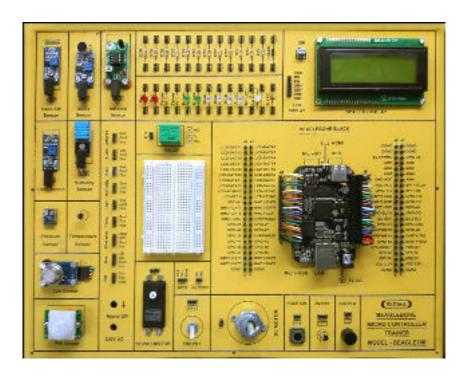
This trainer has been designed with a view to provide practical and experimental knowledge of Internet of Things (IOT) with Sensors programing with BeagleBone Board.
