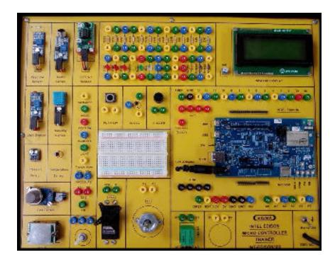
This trainer has been designed with a view to provide practical and experimental knowledge of Internet of Things (IOT) with Sensors programing with Intel Galileo Microcontroller Board.
