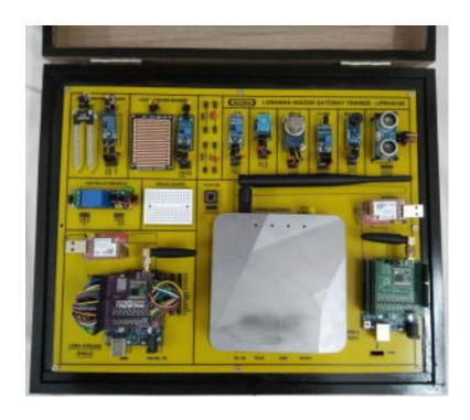
This trainer has been designed with a view to provide practical and experimental knowledge of Internet of Things (IOT) with Sensors programing with Lora Arm Cortex M4 and ESP32 IOT Boards.
