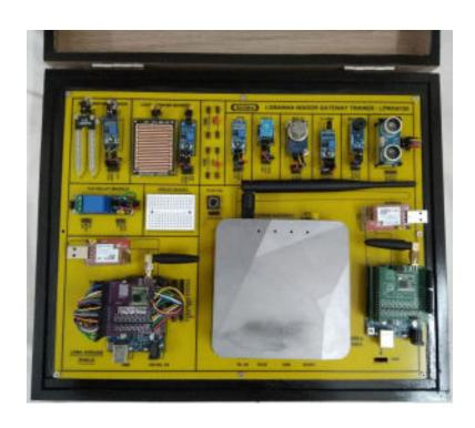
This trainer has been designed with a view to provide practical and experimental knowledge of Internet of Things (IOT) with LoRaWAN Peer to peer Communication Sensors programing with Arduino IOT Boards with LoRaWAN Gateways.
