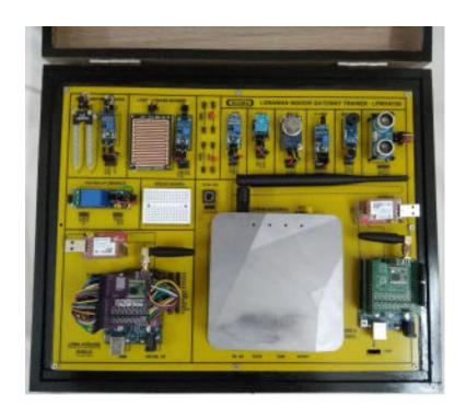
This trainer has been designed with a view to provide practical and experimental knowledge of Internet of Things (IOT) with LoRaWAN Gateway Communication Sensors programing with Arduino IOT Boards with LoRaWAN Gateways.
