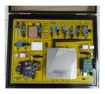
This trainer has been designed with a view to provide practical and experimental knowledge of Internet of Things (IOT) with Sensors programing with ESP32 LoRaWAN IOT Board.
