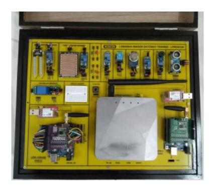
This trainer has been designed with a view to provide practical and experimental knowledge of Internet of Things (IOT) with LoRaWAN Gateway Communication Sensors programing with Raspberry IOT Boards with LoRaWAN Gateways.
