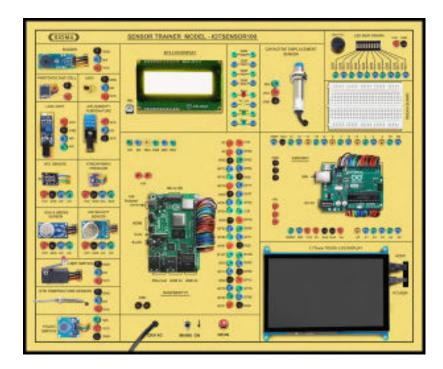
This AI Enhanced IoT Application Setup Trainer has been designed with a view to provide practical and experimental knowledge of Internet of Things (IOT) and Artificial Intelligence (AI, ML, DL and NLP) with Sensors programing with Raspberry, Arduino and Jetson IOT Boards.
