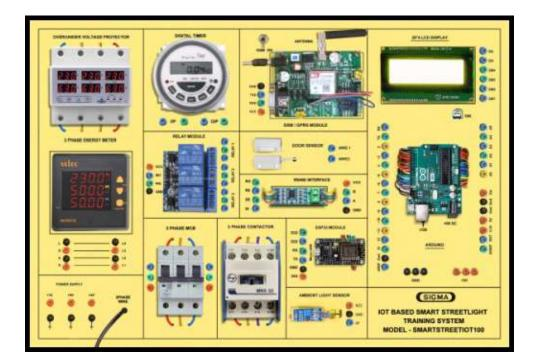
This trainer has been designed with a view to provide practical and experimental knowledge Sensors programing for IoT based Smart Street Light system with Arduino IOT Board.
