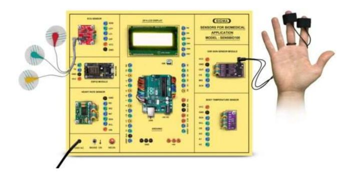
This trainer has been designed with a view to provide practical and experimental knowledge of ECG cum Heart Rate Monitor using Biomedical Sensors programing for Internet of Things (IOT) with Arduino IOT Board.
