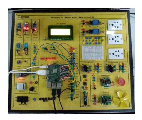
This trainer has been designed with a view to provide practical and experimental knowledge of using Programmable Logic Controllers (PLC), Distributed Control Systems (DCS), Supervisory Control and Data Acquisition Systems (SCADA) with Raspberry Industrial IOT Gateway. IIoT Gateway is reliable open platform for collecting, Processing and transmission data.
