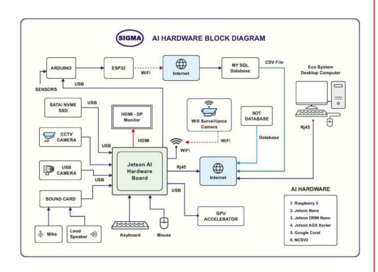
This trainer has been designed with a view to provide practical and experimental knowledge of Natural Language Processing NLP with Artificial Intelligence (AI) hardware and software programing with A57 Microcontroller.
