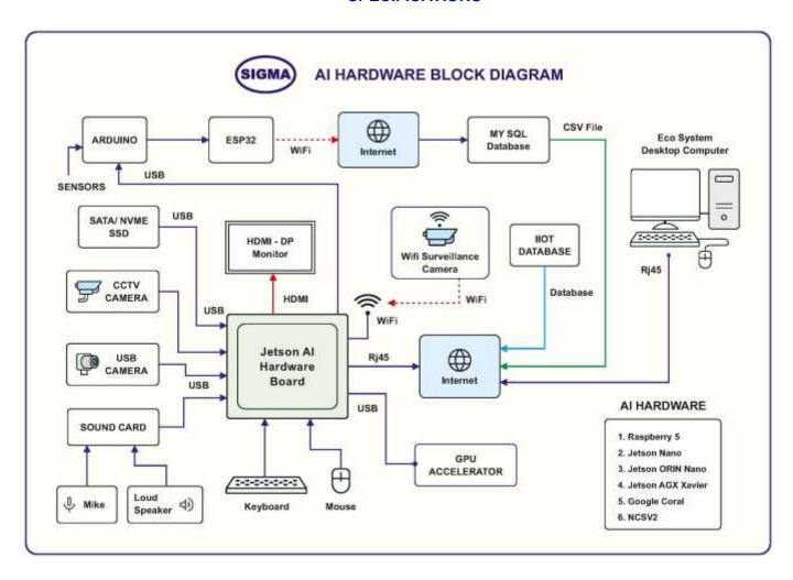
This trainer has been designed with a view to provide practical and experimental knowledge of Machine Learning and Deep Learning Technology using Medium speed GPU AI Board.
