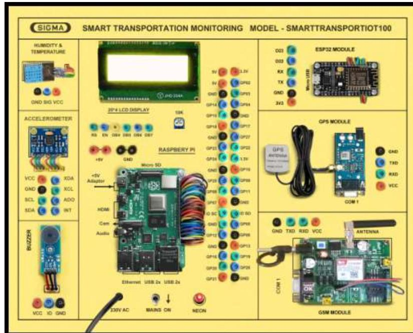
This trainer has been designed with a view to provide practical and experimental knowledge of Sensors programming for Smart Transportation Monitoring System with Raspberry IOT Board.
